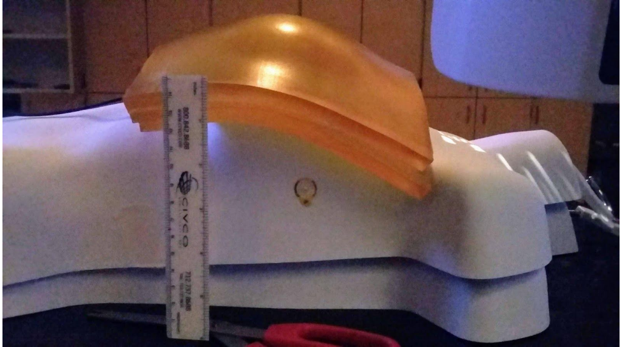
Figure 2: Mannequin setup for the 12E beam. There is 3 cm bolus over the QED. We centered the bolus and QED on the breast of the phantom. The second mannequin is underneath to hold the inner bolus in place. For this setup, the gantry angle was 10 degrees to make this an enface beam.
